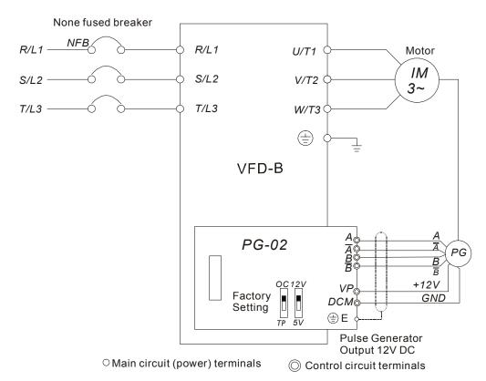
PG-02 and Pulse Generator Connections
