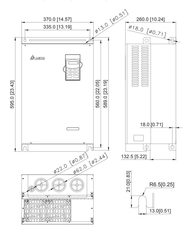
Frame F: VFD550B43A, VFD750B43A
