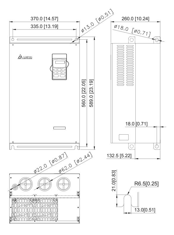
Frame E1: VFD300B23A, VFD370B23A, VFD550B43C/53A, VFD750B43C/53A
