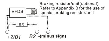
Connect a brake resistor or brake unit in applications with frequent deceleration ramps, short deceleration time, too low braking torque or requiring increased braking torque.
