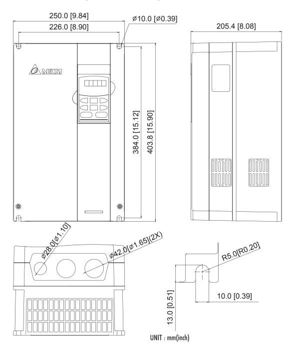
Frame E: VFD300B43A/53A, VFD370B43A/53A, VFD450B43A/53A
