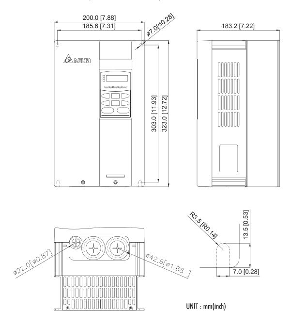
Frame D: VFD150B23A/43A/53A, VFD185B23A/43A/53A, VFD220B23A/43A/53A
