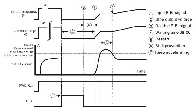
Fig 3: B.B. Speed Search with Minimum Output Frequency Upward Timing Chart
