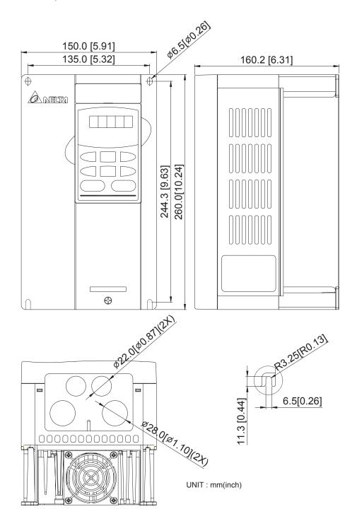
Frame C: VFD055B23A/43A/53A, VFD075B23A/43A/53A, VFD110B23A/43A/53A
