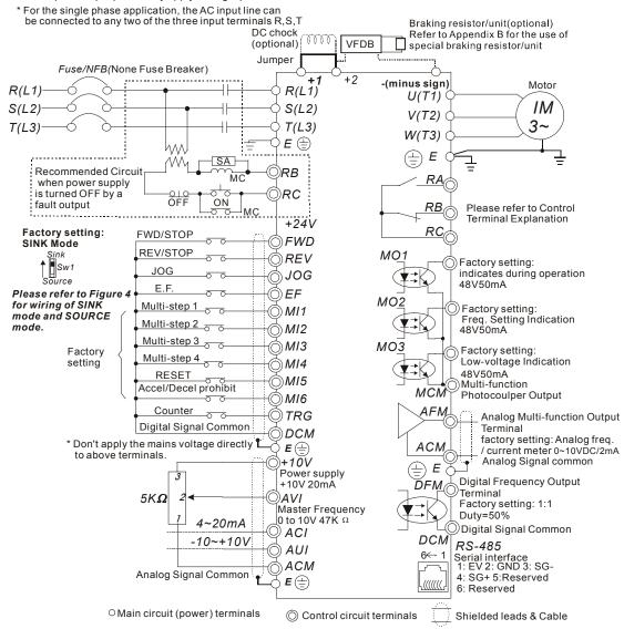
Figure 4 Wiring for SINK mode and SOURCE mode
