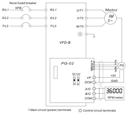
PG-02 and Pulse Generator Connections
