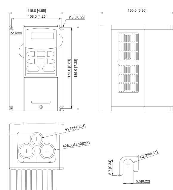
Frame A2: VFD015B21B/23B, VFD022B23B/43B/53A
